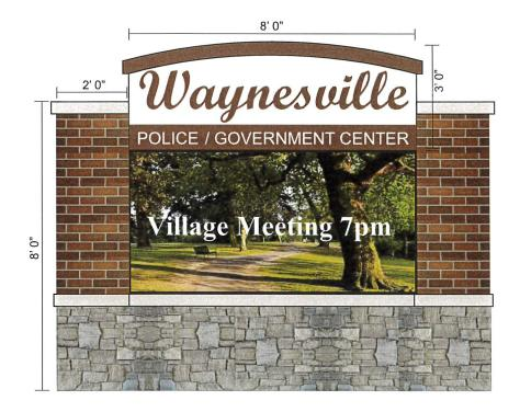
Production and Installation of 8' 0" x 12' 0" Monument Sign. Sign internally illumintaed and double sided. Sign to include Upper Cabinet 3' 0" x 8' 0", reading "Waynesville Est. 1796", with decorative eyebrow. Sign fabricated using 080 aluminum and reverse cut text. Painted Matthews Paint White, and Pantone matched red, flat. Acrlic red text with back lighting.
